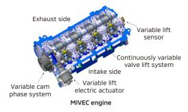
The MIVEC is a variable valve timing mechanism for minimizing fuel consumption. The intake valve lift is continuously varied according to the operating condition to reduce intake resistance. This minimizes air intake energy loss, resulting in improved fuel efficiency.
