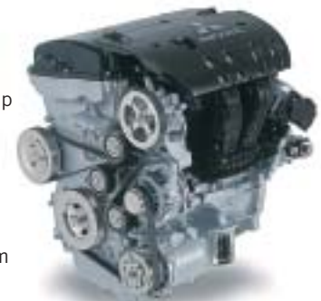
New 2.4 liter, 4-cylinder MIVEC engine fitted on the Outlander
