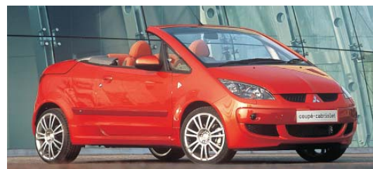
Colt CZC (Coupe Cabriolet model) Derived from the three-door Colt CZ3, this cabriolet model is equipped with an automatic retractable roof. Produced in Europe, it is the third in a series of body frame variations following the Colt five and three-door models. Scheduled for roll out in 2006.
